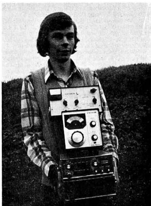
A complete portable station in the palms of two hands (those of G8ILI, son of G3FDW). The equipment, top to bottom, is a Europa 4 transverter, a vfo for 70MHz, FT75 ssb source, and its psu. GM3FDW/P will activate Border counties on 4m from 1 to 7 September. (Photo by G3FDW.)
